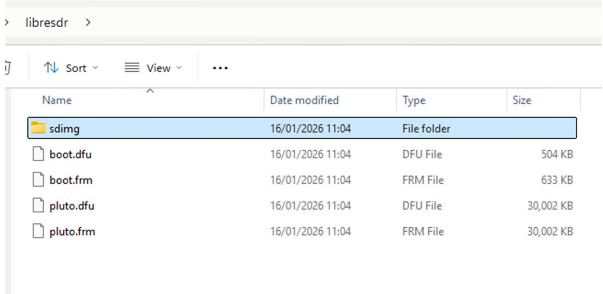
**Copy Files to the SD Card:** Copy the boot.dfu, boot.frm, pluto.dfu and pluto.frm to your prepared SD Card.
