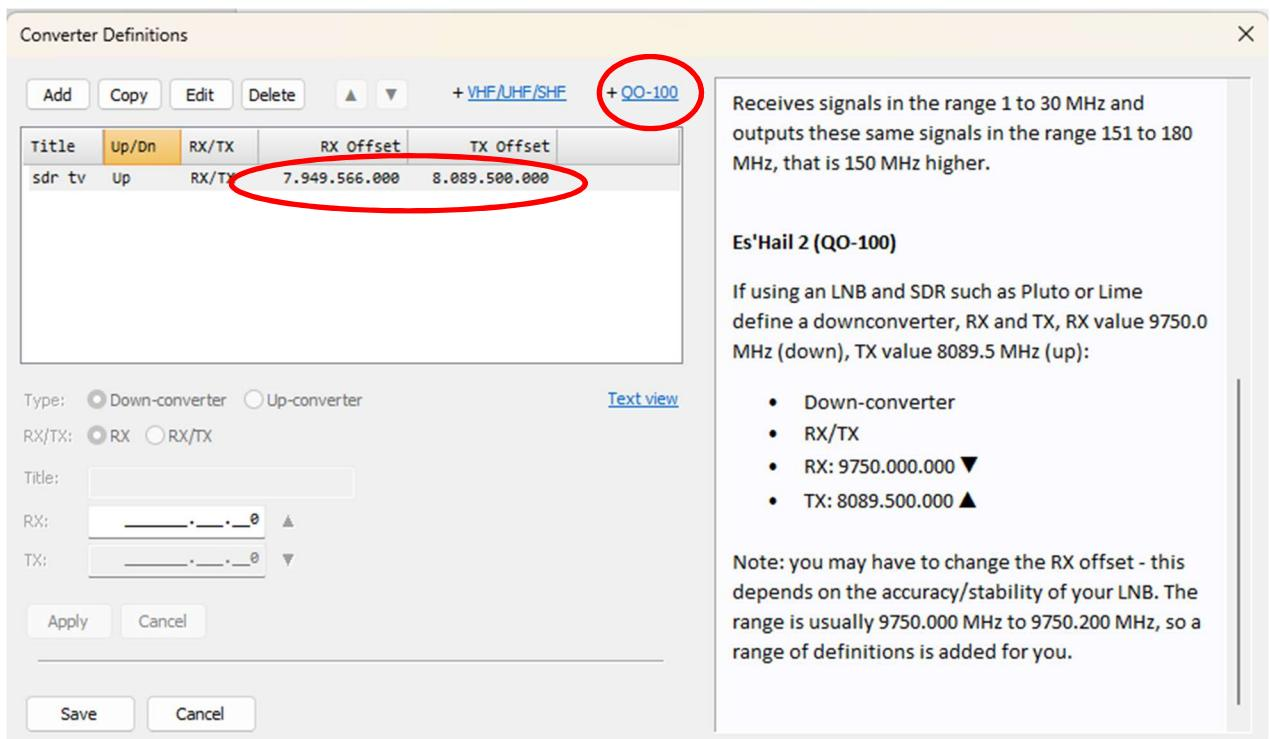
Please note that the transmission from the satellite uses horizontal polarization so you will need to provide the LNB with 18 Volts via a Bias-T
